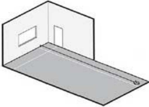
**2. Loose lay** - Loose lay the tiles (without adhesive) starting along the centrelines and following the arrows printed on the back of the tile taking special care to the alignment of joints and/or pattern. The loose laying is very important in order to check the colour uniformity and the absence of defects of the flooring. Claims for defects can only be investigated prior to fitting the floor.
