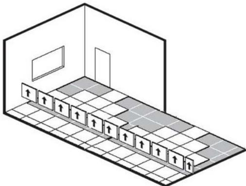
**3. Cutting** - Check the uniformity of colour and the absence of defects. The perimeter tiles should be trimmed off ready for bonding.
