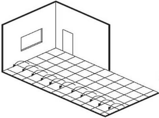
**6. Bonding** - When using adhesive with long tackifying time, applying weights along the joints (bricks, sand bags, etc.) will help with the bonding process.
