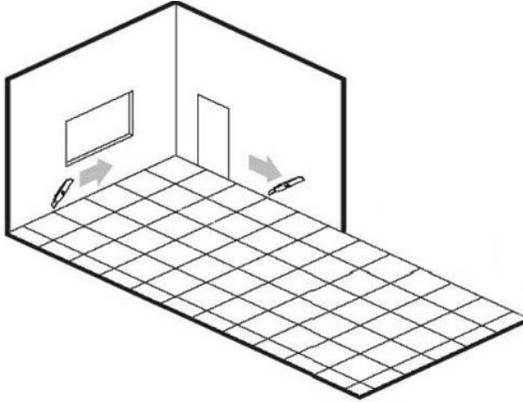
**4. Adhesive** - Tip over a row of tiles at a time. Spread the adhesive with the proper notched trowel as advised by the manufacturer.
