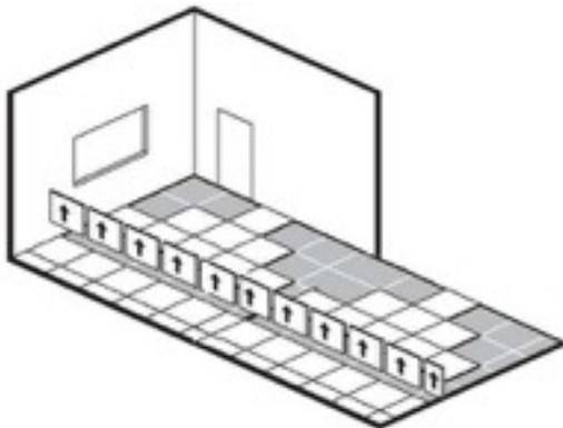
**3. Cutting** - Check the uniformity of colour and the absence of defects. The perimeter tiles should be trimmed off ready for bonding.
