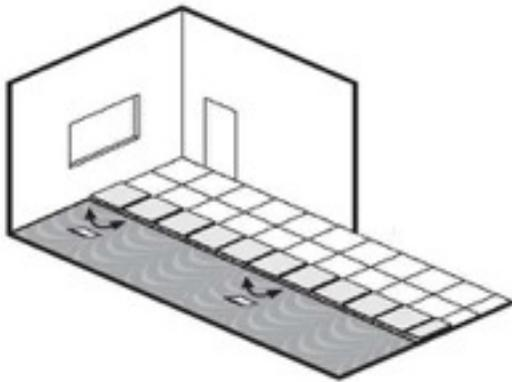
**5. Fitting** - Once the adhesive is ready to accept the tiles, put the tiles back in the starting position. Press/massage the flooring to make sure that all air is expelled and the tile is in full contact with the substrate. Special care has to be taken with regards to the positioning of the tiles to make sure the alignment of joints and studs is accurate.
